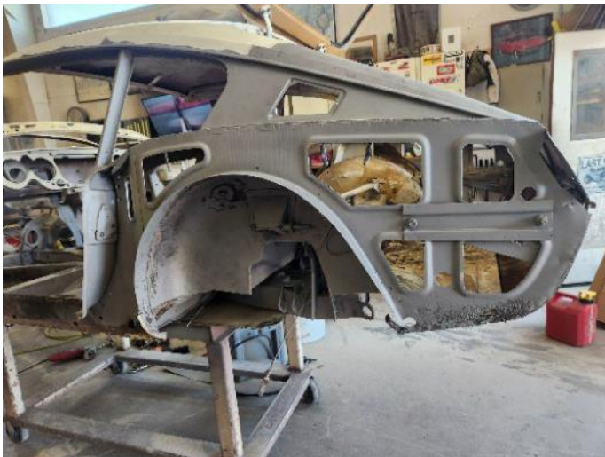
This picture shows metal body panels that were purchased and in place.
