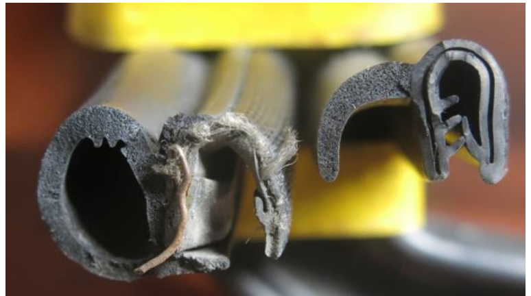
Old door seal on left, MacGregor's seal on right
