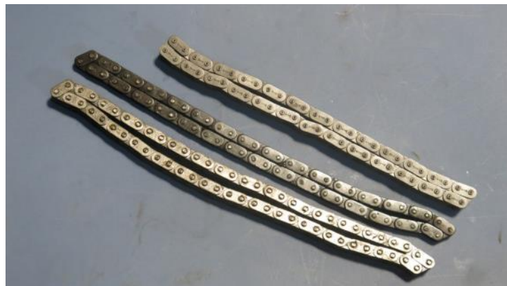
From top to bottom: Wrong duplex chain, original chain and new duplex chain
