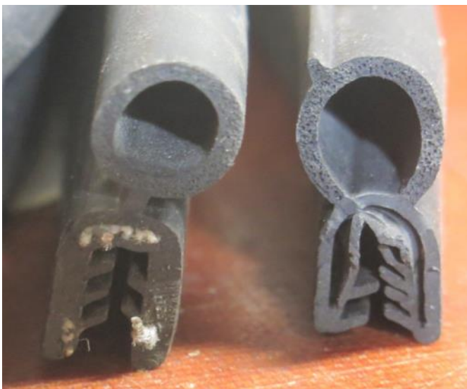
First hatch seal on left. MacGregor's seal on right
