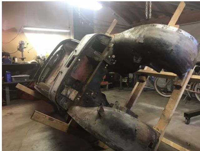
DIY wood frame to flip tub side to side
