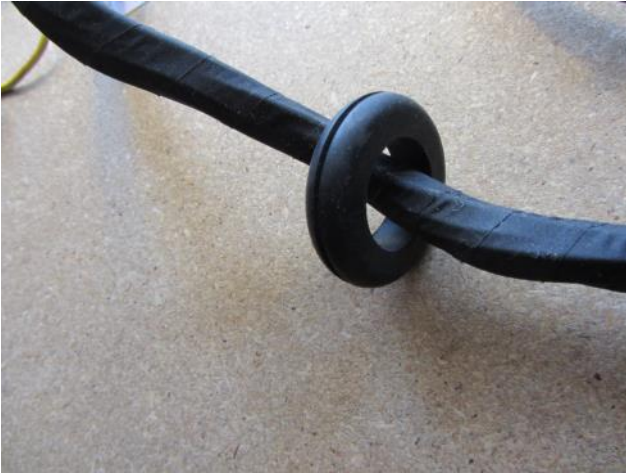
New firewall grommets need to be in place before wrapping
