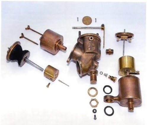
The bespoke set-up of twin vertical dashpot downdraught carburettors of unique design which were manufactured by the SU Company specifically for the MG 18/100 Mk III 'Tiaresse'. (Author)
