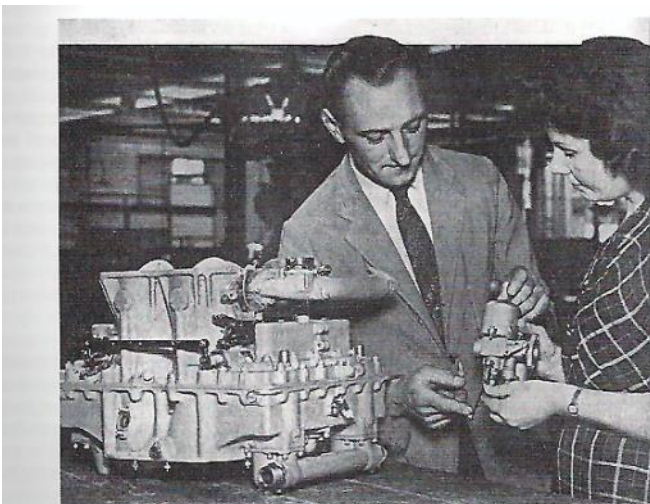
Publicity photograph showing the difference in size between an SU aero-carburetter and an SU vehicle carburetter. The aero-carburetter is a four-barrel Napier-Sabre II unit. (Reproduced from 'Calling All Arms')
