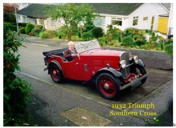
considered the Southern Cross to be the first real Triumph Sports Car. It certainly looked the part: open four seater with tonneau often covering the rear seats, cycle fenders, folding windshield, Brookland steering wheel, full instrumentation including tachometer, spare mounted at the back and wire wheels. *Autocar* magazine had this to say: "A car which will have strong appeal to the sportsman. A sports car with considerable refinement in its running".
