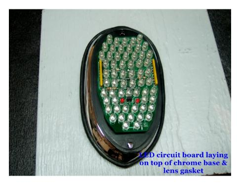
3. Take the chrome lamp base to the workbench and drill out the 2 rivets securing the bulb holder. I used a 5/64th drill bit which leaves the base unblemished in the unlikely event you would some day want to remount the bulb holder and return to the incandescent bulb. The circuit board will now have room to lay on top of the lens gasket and be held in place by the lens.
