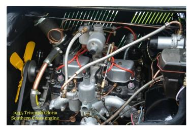
All Glorias were powered by Coventry Climax designed overhead intake and side exhaust 4 & 6 cylinder engines. They were well equipped cars with permanent jacking systems, windscreen washers, self canceling turn indicators, tachometer, clock and optional metallic paint. Other options
