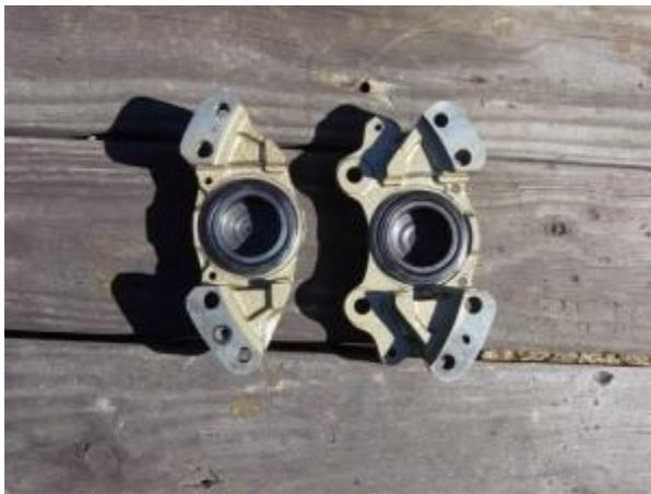
Bolt the mess back together. Unbolt it and place the little seal that you forgot between the halves. Bolt it back together again and torque all bolts to 2½ grunts. Might as well paint it before reassembling on the car, which is more or less the reverse of what you did previously.
