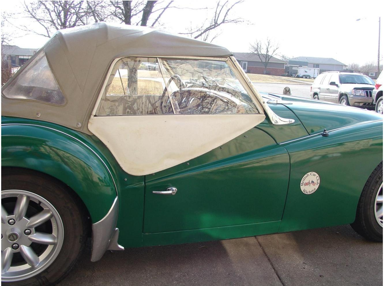
One final note, if you have the original plexiglass windows in your car, the front plexiglass is sewn into the vinyl instead of glued. The front plexiglass is very thin and can be sewn with a good sewing machine or by hand.
